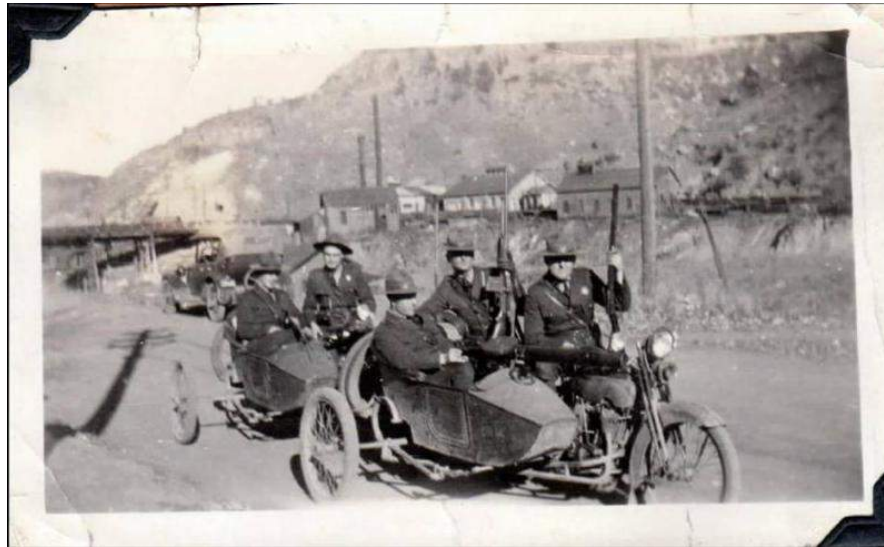
As seen in this picture, the extended wheels of the sidecar provided stability while driving in wagon ruts. Mounted in the sidecar is a drum-mounted machine gun.
