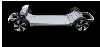
Faraday Future chassis with battery between axles
